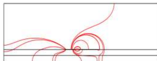
Figure 5. Streamline plot of asymmetric coupled microstrips on a two-layer substrate.
